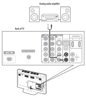
3 Turn on your TV, then turn on the analog audio amplifier and set it to the correct output mode. See the documentation that came with the amplifier for more information.
